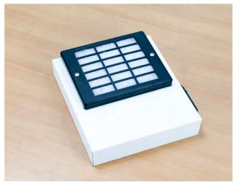
2a. Attach the Ventilation–unit to the Lower Back-cover, on the **inside**
