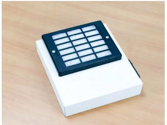
Attach the Ventilation–unit to the Lower Back-cover, on the <u>outside</u>.
