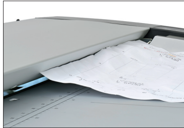
Funnel-shaped feed handles torn and wrinkled documents with ease.
