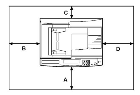
Over 750 mm (29.6") A: In Front: Over 100 mm (4.0") B: Left: C: Rear: Over 100 mm (4.0") D: Right: Over 100 mm (4.0")
